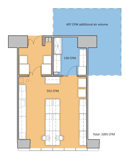
A 6' fume hood consuming 543 CFM in an enclosed support room exceeds the minimum exhaust air requirement and additional air volume is required
